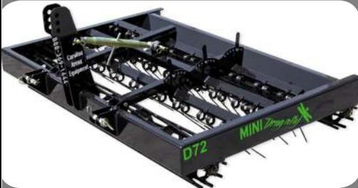
The MINI DragNfly has an open cage roller on the front, next there is three rows of tines that work like fingers to mix and spread the surface keeping the footing from clumping, giving an ultimate mixing effect of the surface. This drag is designed to mix the surface only. This drag cannot dig, working great for shallow footing surfaces. It can be pulled behind ATV, golfcart etc, or small compact tractor.
